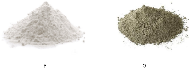
Fig. 6. Ciment alb (a); ciment gri (b)
